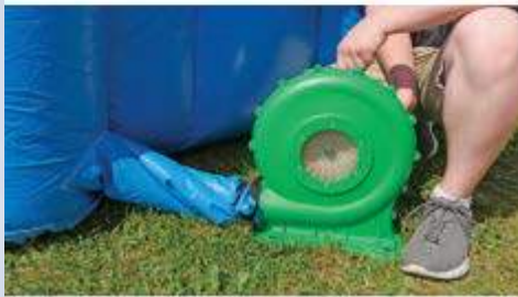
A twisted air portal will severely restrict air flow.
